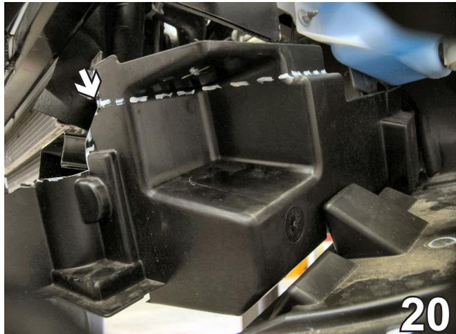
20. On the driver's side, approximately one inch from the top of the air dam, cut horizontally from the front of the air dam to the back.
