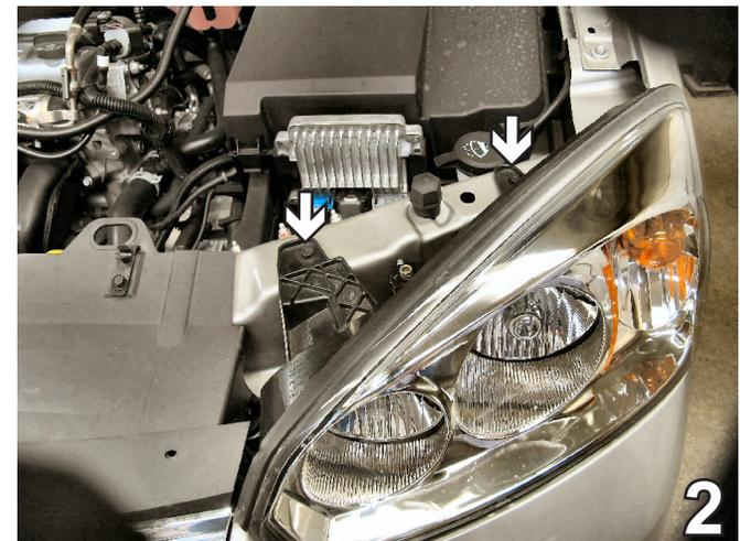
2. Using the 10MM socket, remove two metric bolts from the headlight assembly. Pull the headlight assembly forward and disconnect electrical connections. Do this to both sides of the vehicle. Set bolts and headlight assemblies aside to reinstall later.
