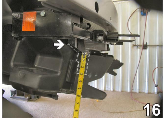
16. Mark the passenger's side of the air dam from the front portion of lip diagonally to the bend and down 3 inches around the contour of the air dam mold. Then mark straight down from the air dam tab three inches and horizontally back to the air dam contour and trim this area with the utility knife.
