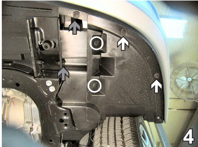
4. Using the 7MM socket, remove two metric bolts from underneath corner of the front fascia, forward of the front tire, as indicated by the white arrows in the photo above. Remove two Christmas tree pushpins, as indicated by the circles in the photo above. Remove two pushpins, as indicated by the grey arrows in the photo above. Do this to both sides of the vehicle. Set bolts and pushpins aside to reinstall later.
