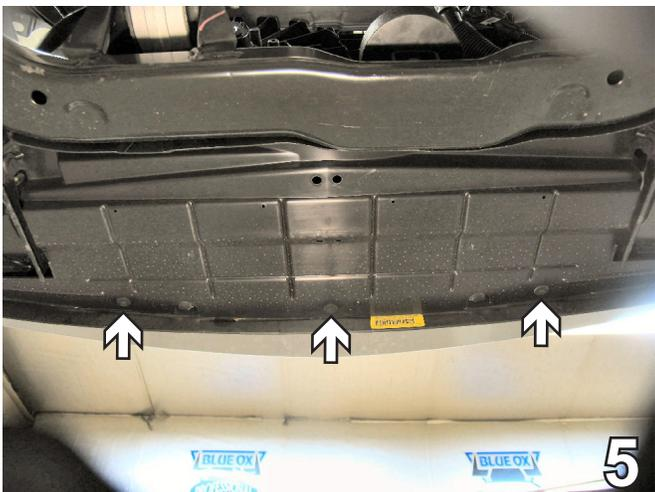
5. Using the 7MM socket, remove three metric bolts underneath the fascia. Set bolts aside to reinstall later.
