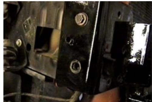
9. Align the baseplate with existing holes on the outside of passenger's side frame rail and tighten the two existing bolts. Clamp baseplate on driver's side to align with top edge of frame rail with the vise grip. **Be sure and use loctite on all bolts before tightening. Torque all bolts according to Torque Chart in General Instructions.**
