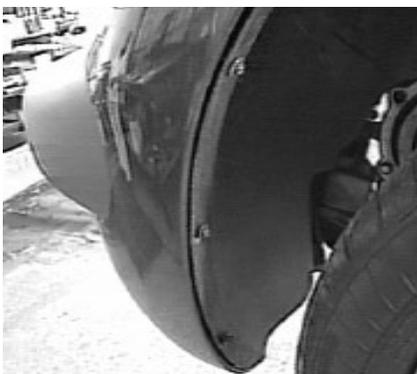
3. Just forward of front tires are three metric bolts to remove on wheel well with the 10MM socket, both sides.
