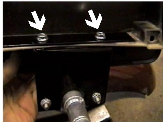
**15.** Reinstall front fascia and remove license plate bracket using the 10MM socket. Using item 8 as a template, center and drill two holes into the bottom of license plate bracket with the 9/32" drill bit. Install items 8, 10, 11, 12 and 13 to license plate bracket according to drawing on last page. Reinstall license plate bracket.
