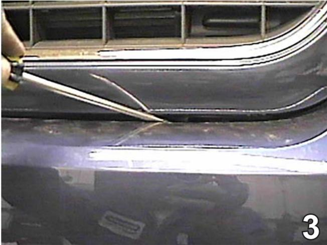
3. There is a slot under each headlight and three under the grille assembly that join the bumper fascia. Insert a flat head screw driver and pry down while pulling the fascia forward. Set the headlight assemble aside to be reinstalled later.
