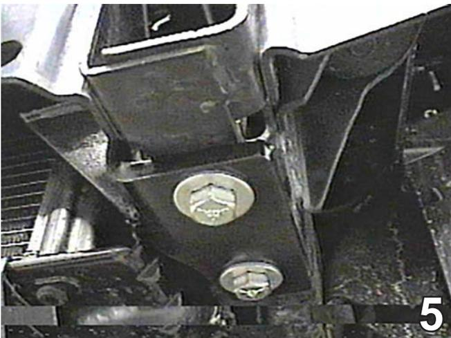
5. Hold the baseplate into place and align with the existing holes on the bottom side of the frame. Install the 1/2-13 x 1 3/4" hex washer, 1/2" lock washer, and the 1/2" flat washer. Then insert the 1/2-13 nut plate into the frame end. (See **LOCTITE** note)
