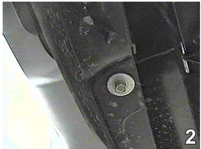
2. Using a 10MM socket remove two metric bolts with 10MM socket and push pins on the bottom side of fascia. There is a (the 2005 models have two) 10MM bolt to remove inside the wheel well. Do this to both sides of the vehicle. Set the metric bolts aside to be reinstalled later.
