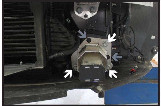
6. Remove the two (2) push pins from the brace (gray). Using a 15MM socket remove the three (3) bolts from brace (white). Do this on both sides of vehicle. Set aside the bolts for installation of baseplate, the brace and push pins will not be reused.
