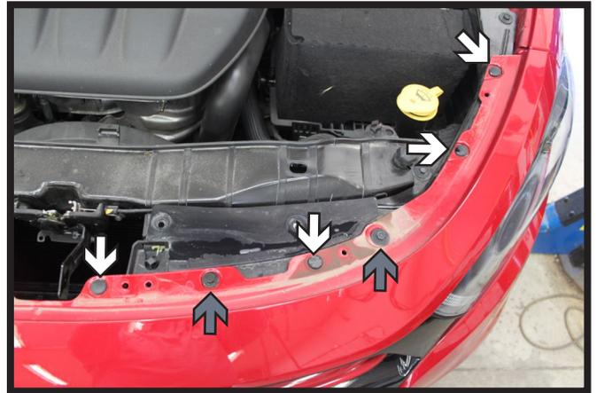
2. On top side of fascia, remove the four (4) push pins (white). Using a 10MM socket, remove the two (2) screws (gray). Do this on both sides of vehicle.
