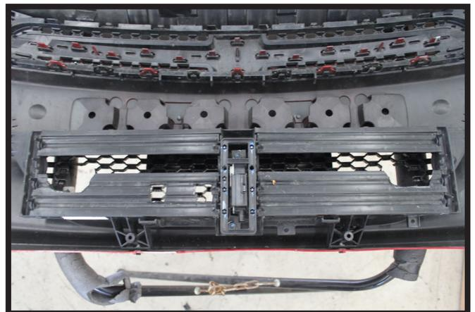
11. On both sides of the shutter, trim the remaining shutter blades as needed to fit around the attachment tabs and electrical rods.
