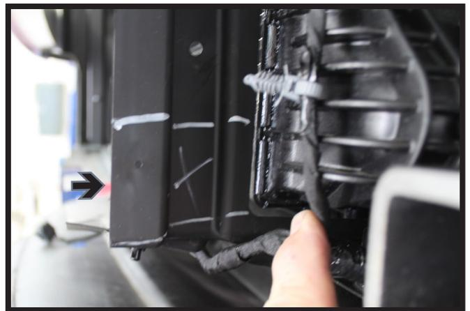
7. Trim the plastic shrouding in front of radiator on both sides of the vehicle approximately as shown for clearance of the baseplate installation. Further trimming may be required until baseplate clears the shroud.
