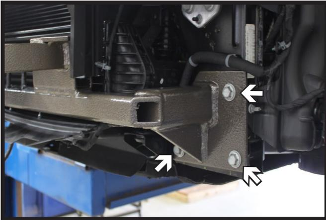
8. Attach the baseplate to vehicle using the six (6) existing holes and bolts. Be sure to use Loctite® Red on threads before tightening.
