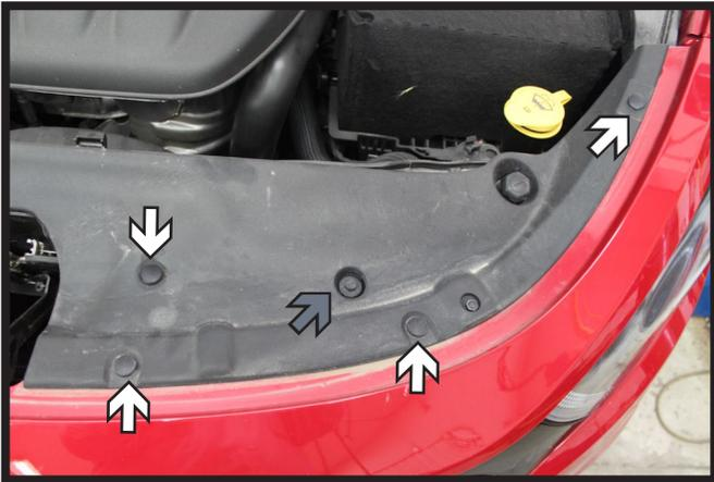
1. Remove the four (4) push pins (white). Using a 10MM socket, remove the one (1) screw (gray). Do this on both sides of vehicle. Remove the top cover and set aside.
