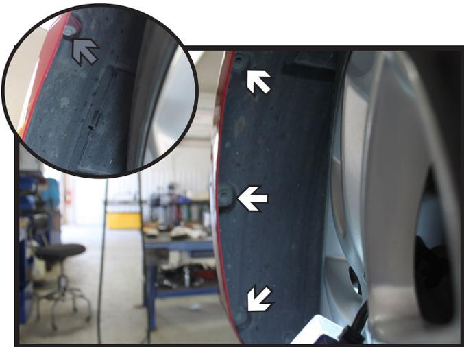
3. Using a 10MM socket, remove the one (1) upper screw from wheel well (inset). Using a 8MM socket remove the lower three (3) screws from wheel well (white). Do this on both sides of vehicle.
