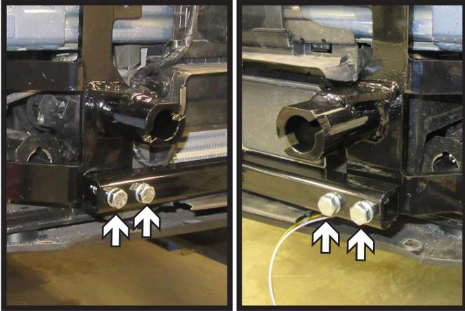
17. Using four (4) 1/2" x 2-3/4" bolts with lock washer and nylon lock nut attach the center cross bar to the side plates. If the holes do not completely line up, ream out holes with a drill bit.
