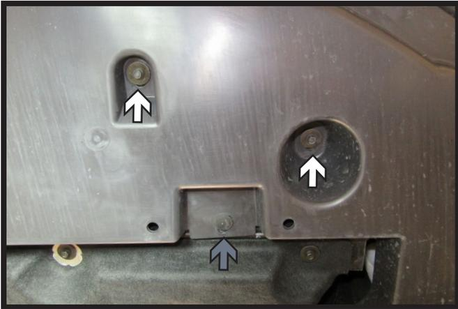
7. Using a 7MM socket remove the two (2) bolts (white) and one (1) push pin (gray) from the belly pan. Do this on both sides of the vehicle. Remove belly pan.
