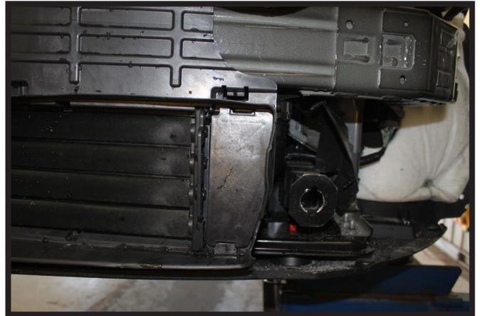
7b. **Shutter Models without ACC Only:** Remove the shield on the driver side next to the shutter support.
