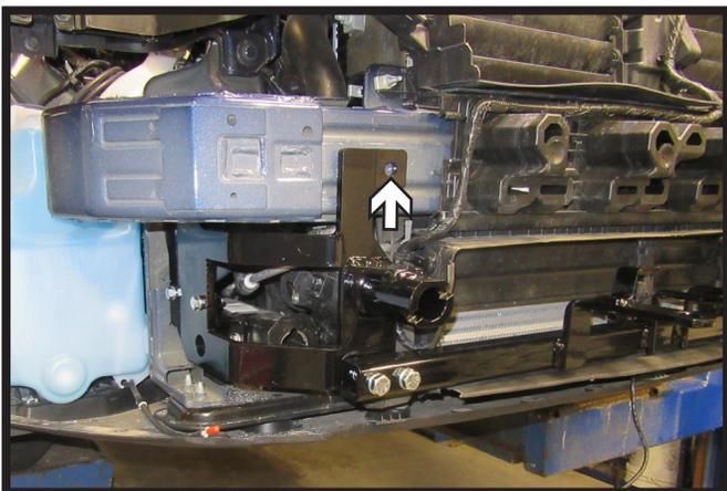
19. Insert one (1) 1/2" bolt with spacer on the back side. If the spacer cannot be attached perfectly up and down, may need to angle spacer slightly to get it to fit. Do this on both sides of the vehicle.
