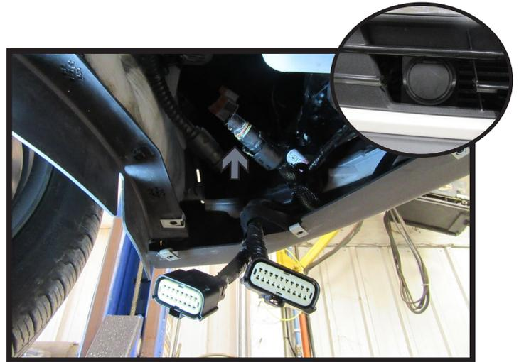
8. Unplug electrical cable on the underside of the fascia. If the vehicle has a plug on the passenger side of the vehicle as shown in insert, will need to unplug the engine block heater as indicated (gray) and remove. Then remove the fascia.
