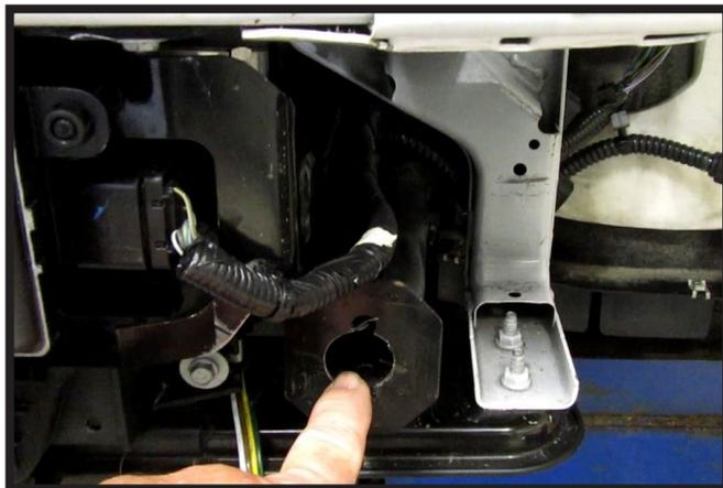
17. Using a 1-1/4" drill bit drill one (1) hole as indicated. Do this on both sides of the vehicle.
