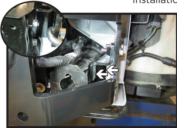
23. Before attaching the safety cables drill out bottom two (2) indicated holes using a 3/8" drill bit. Then insert two (2) 3/8" bolts with lock washers. Do this on both sides of the vehicle.
