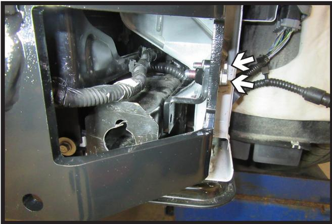
19. Using two (2) 3/8" bolts attach the Z bracket to the side plate as indicated.
