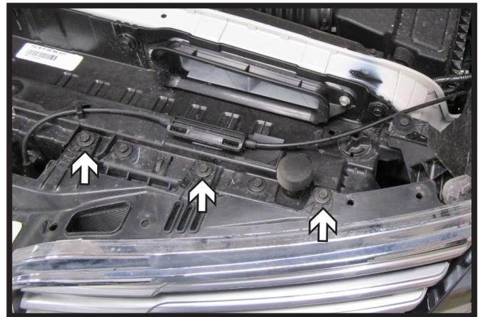
3. Using a 10MM socket remove the three (3) bolts from the top of the fascia. Do this on both side of the vehicle.
