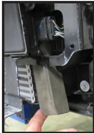
15. Remove the indicated foam pieces from both sides of the vehicle.
