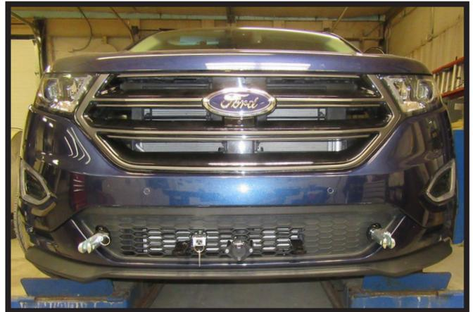
22. Hold the fascia as close to its original position, mark and trim the fascia around the attachment tabs. Reinstall the fascia and fascia cover. Make sure to reconnect all electrical connections.
