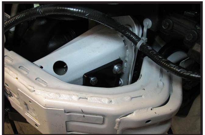
18. Hold up the side bracket and start the top two (2) 3/8" bolts. Use a lock washer with the front bolt. For the back bolt use a flat washer and a lock washer. Make sure the bracket is level and tighten. Do this on both sides of the vehicle.
