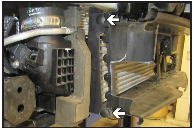
16. Remove the two (2) push pins and then remove the back plastic piece to allow baseplate to fit.
