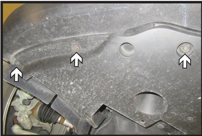
6. Using a 5.5MM socket, remove the ten (10) bolts from the underside of the fascia. There are three (3) on each side and four (4) in the middle. Pull the corners of the fascia away from the vehicle disconnecting any electrical connections and set the fascia aside to be reinstalled later.
