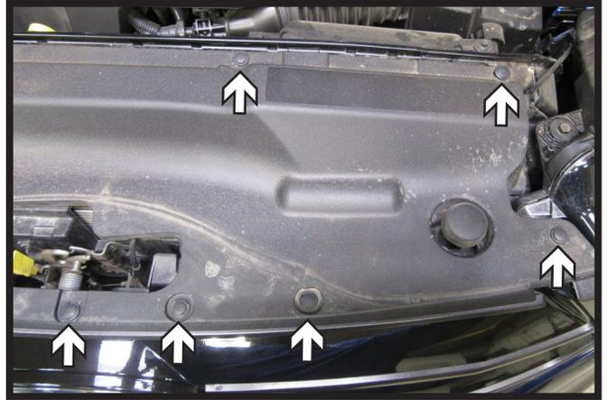
1. Remove the twelve (12) push pins along the top of the fascia cover. Set fascia cover aside to be reinstalled later.
